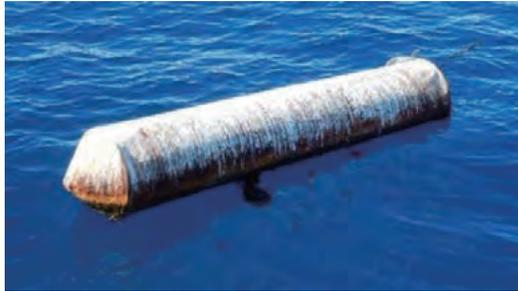
人工浮き漁礁 FAD (Fish aggregating device)
