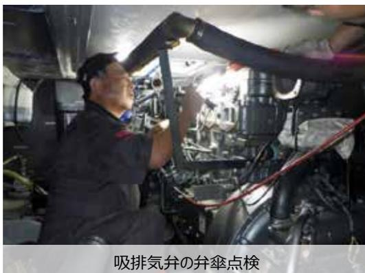
吸排気弁の弁傘点検
