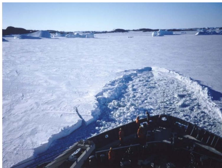
Pic. 1-19: Pulverized ice after crushing by ramming (courtesy of Seiji Shigehara)
