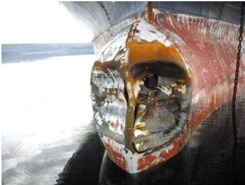
Pic. 3-15: Damage to a bulbous bow from ice load (Source: Website of the Canadian Coast Guard)
