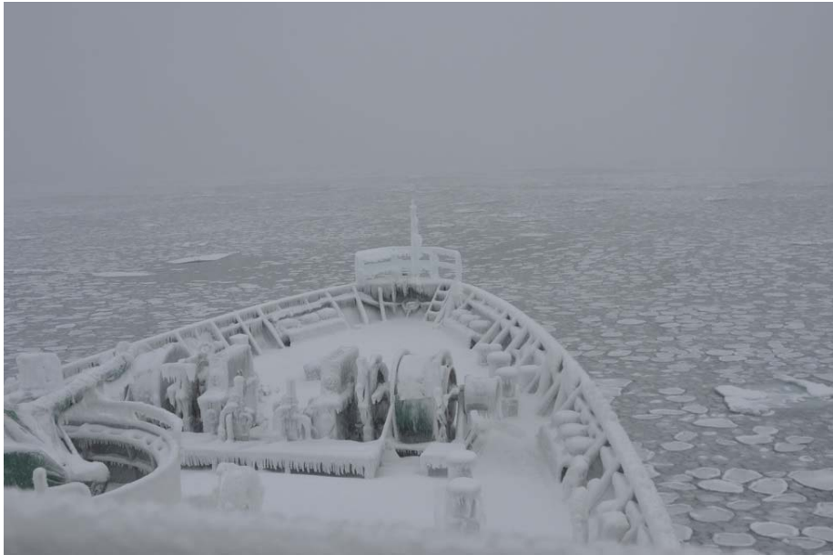
Pic. 2-26: Icing on the bow (courtesy of Kazutaka Tateyama)
