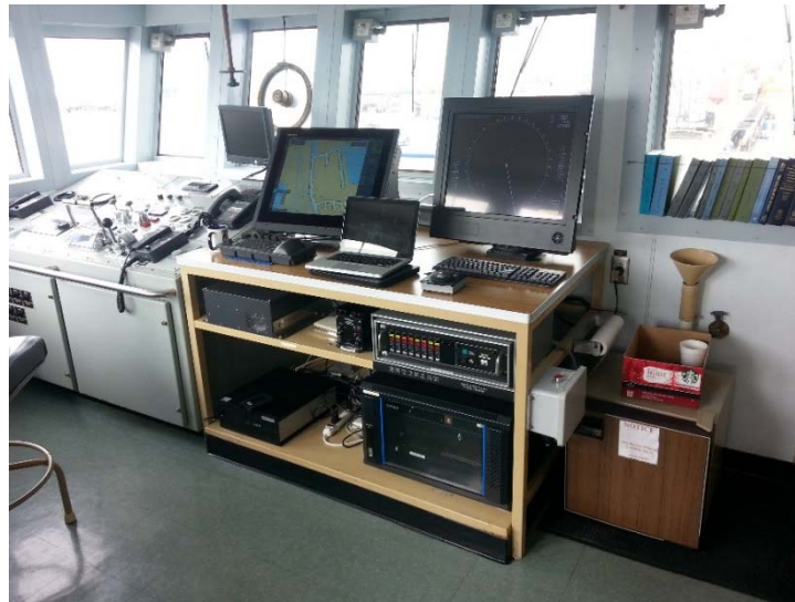
Pic. 2-18: Example of processing equipment installation for sea ice (courtesy of Furuno Electric Co., Ltd.)
