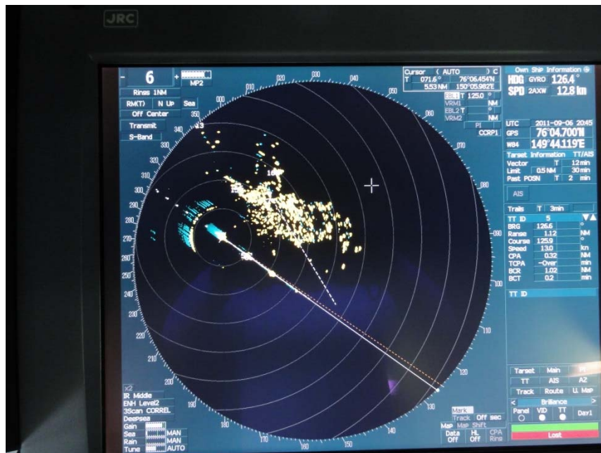
Pic. 2-16: Ice image captured by radar (courtesy of Jin Saijo)
