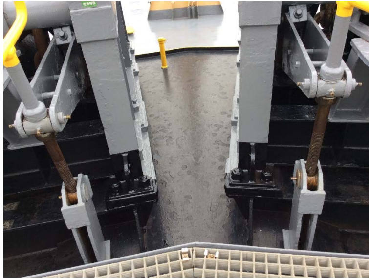
Photograph 2-2-8 When operating the windlass, ensure that the plug is fitted to the oil pan to keep it dry
