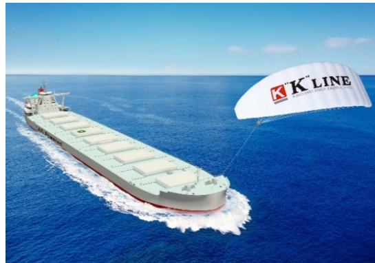
Source: Provided by Kawasaki Kisen Kaisha Ltd. Illustration of a ship with automated kite system
