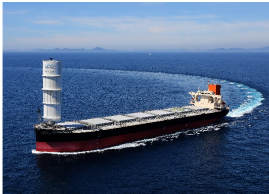
Source: Provided by Mitsui OSK Lines/Tohoku Electric Power Shofu Maru bulk carrier with hard sail propulsion system
