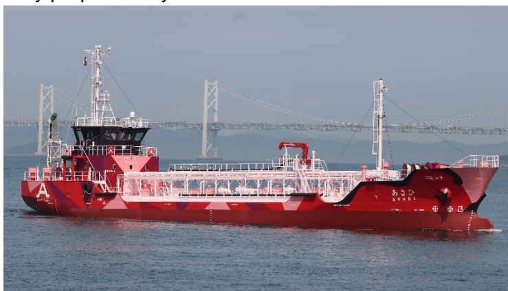
Asahi, an operational electric tanker (March 2022)
