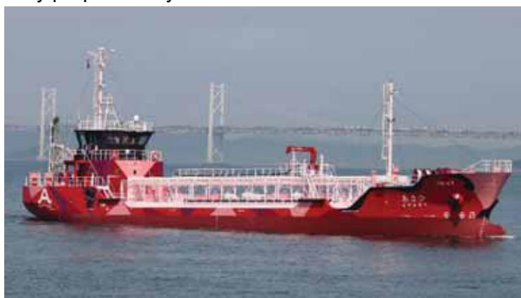
Asahi, an operational electric tanker (March 2022)
